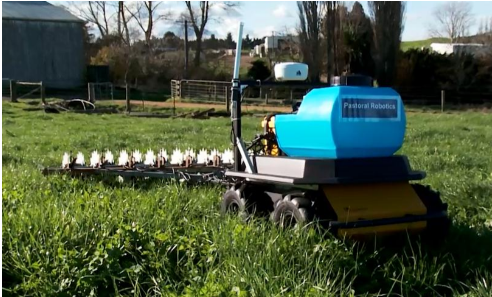
Figure 8. The Mini-ME® autonomous robot towing Spikey®.
